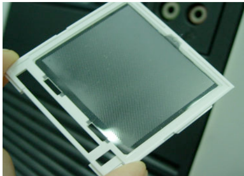
Fig 7: Moulded polycarbonate lightguide for backlighting an LED display. The micro-dot pattern can be seen on the surface. The dots are in the order of 20-150 \mu m diameter. Dot quality, size, and pattern design are critical to the performance.
