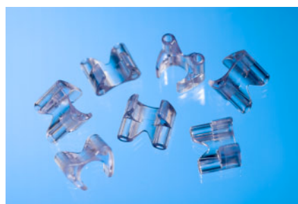
Fig 2: Clip for fluid delivery. The part features a 0.32mm dia hole at a compound angle, formed in the mould by an 11mm long retractable pin.
