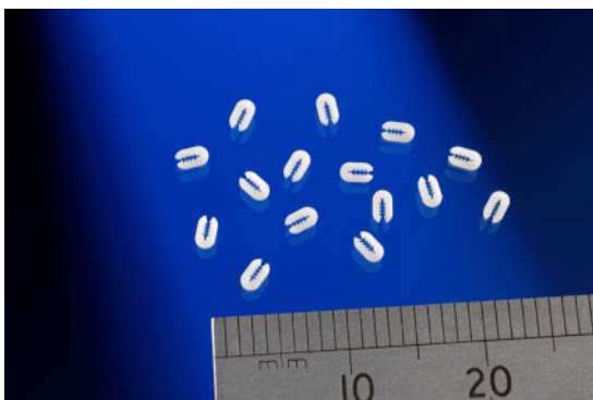
Fig 1: Micro-moulded part for a medical staple. The pitch of the teeth is 0.3mm.
